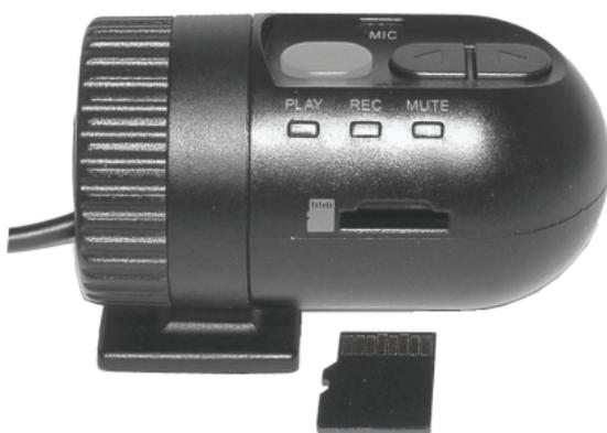
1. Insert the Micro SD card with the text on the card facing DOWN and the electrical contacts facing upwards and inwards.
