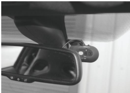
The adhesive mount supplied with the camera uses a VHB 3M adhesive pad. Remove the red sticker from this mount.
