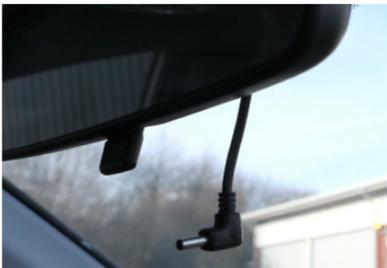
6. Run the cable around the side of the dashboard and underneath towards the cigarette lighter socket. Use cable ties to hide any remaining cable behind the dash.
