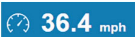
Just below the main video window is the speed of the vehicle shown by default in MPH. Clicking here will change the display to KPH and vice versa.
