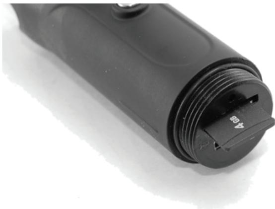
1. Insert the Micro SD card with the text on the card facing UP and the electrical contacts facing downwards and inwards.
