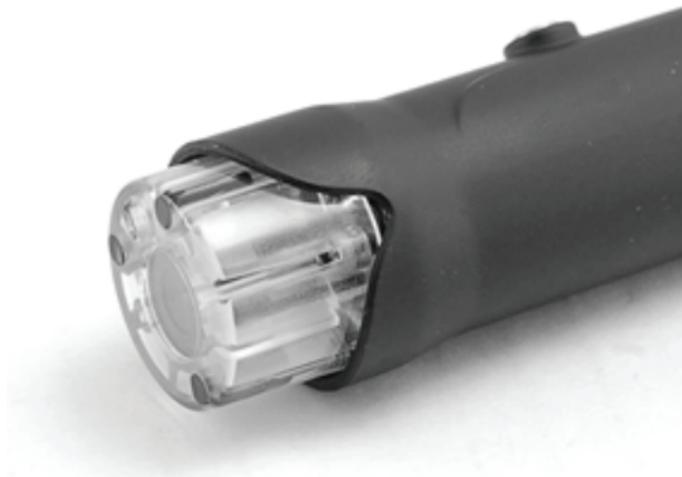
1. The camera has three small coloured LEDs positioned at the front of the camera near to the lens.
